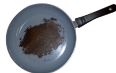
Ceramic frying pan after 1,000 abrasion cycles
